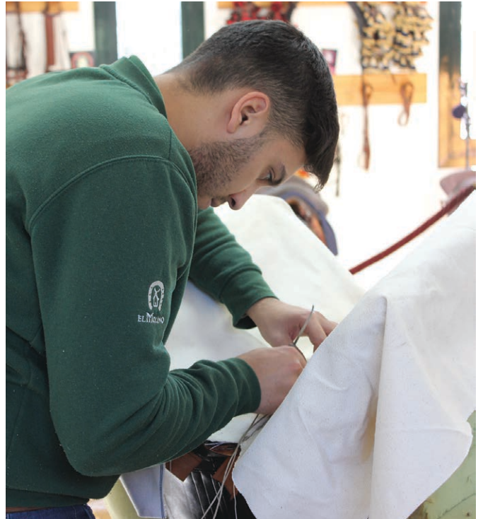
(ABOVE) An apprentice hand sewing part of a Spanish saddle.
